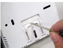
1. Insert flat head screwdriver into position as shown.
