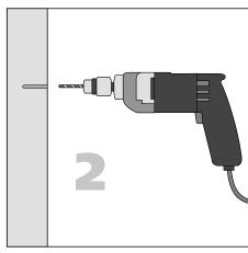
2. Drill holes with the 5mm ø drill bit the length of the supplied dowel plug (30mm deep).
