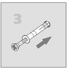
Insert the supplied screws part-way into the plugs. Place dowel and screw into hole drilled into wall.
