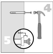
4. Hammer nail into wall. 5. Leave 5mm of the screw protruding out of the wall. This is for the frame to hook onto.
